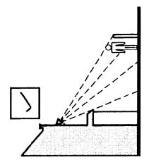
Floodlights and detectors should be aimed to only detect and light people on your property. They should not detect a person or animals walking down the street. If the floodlight is fitted with a timer, this should be adjusted to the minimum to reduce the operation of the light.
