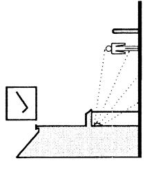
Besides being cheap to run, this type of light is kinder to the environment providing a gentle wash of light with reduced glare. Bulkhead and porch lights cast fewer shadows reducing the hiding places for criminals. These units can be fitted with a movement detector if required. These units are generally mounted lower and are therefore less susceptible to nuisance switching and complaints from neighbours.
