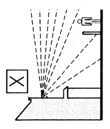
Movement detectors can be useful if they are correctly installed and aimed. Unfortunately, many systems do not allow the detector to be separately aimed from the floodlight.
