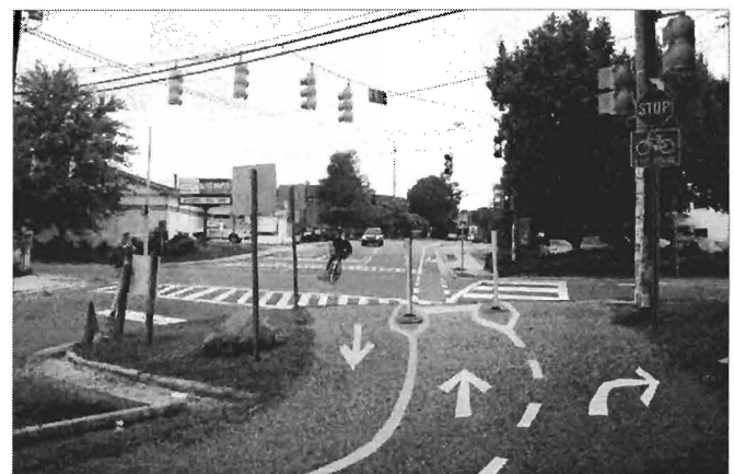
Fig. 3-23. The PTA bike path and Main St./Jones Ferry Rd. intersection is very much in need of improvement. Constructing a turn lane on the bike path would discourage bicyclists from using the sidewalk along Main St.
