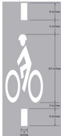
Figure 9C-7. Bicycle Detector Pavement Marking
