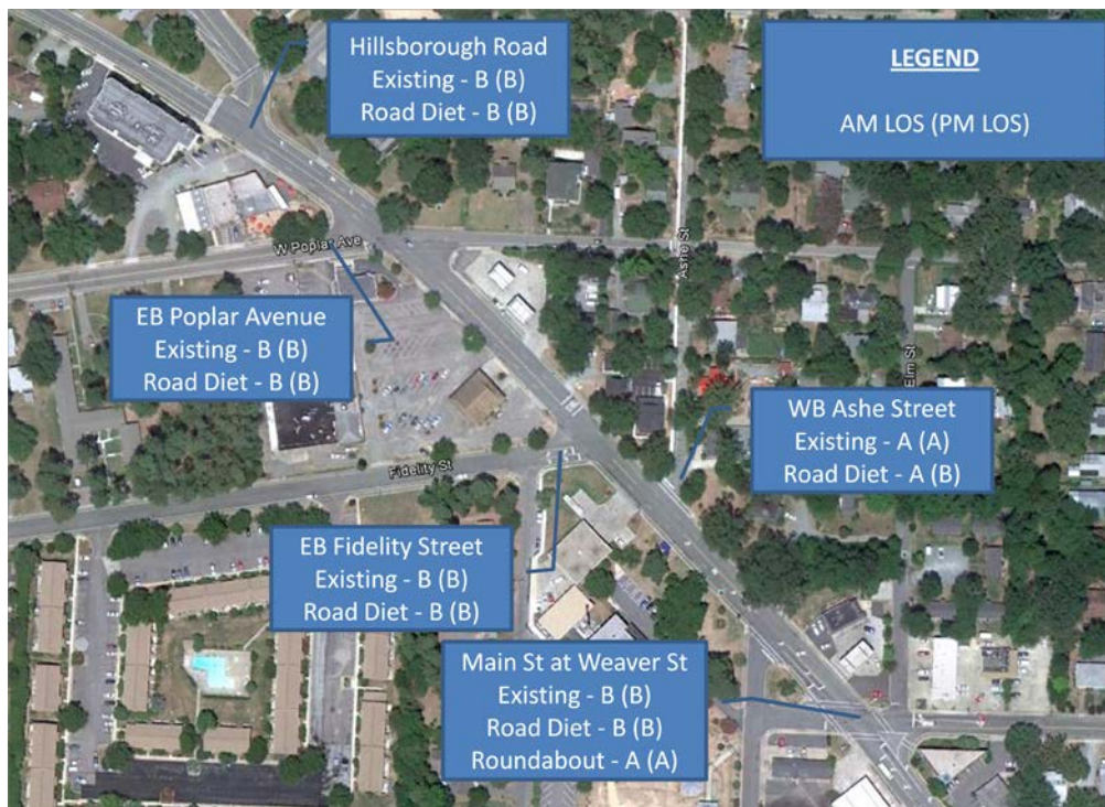
Figure 12: Level of Service Analysis
