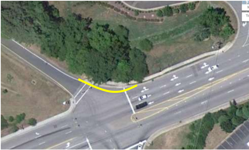
Figure 9. Aerial view of Jones Ferry Rd. at the NC-54 westbound on-ramp with conceptual sketch of sharpened curb radius.
